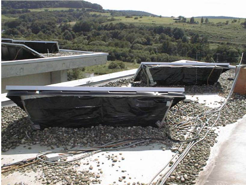
Fig. 10: test system troughs, completely taped up with black foil.
