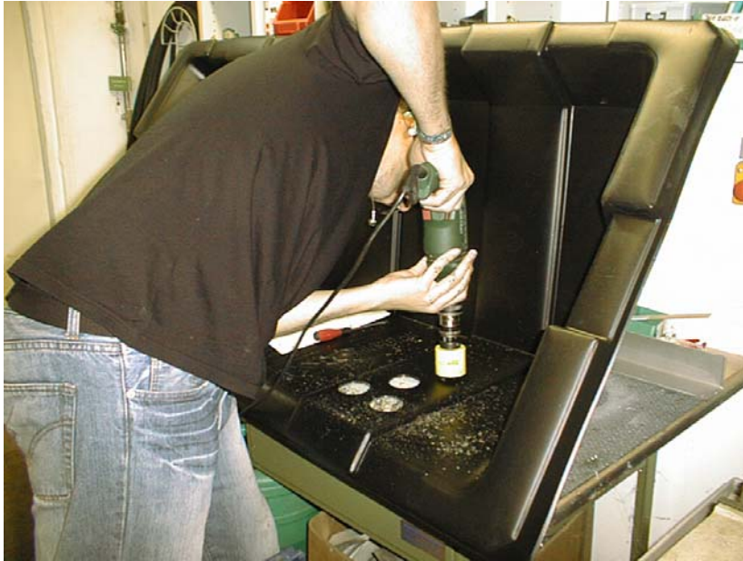
Fig. 3: drilling of ventilation holes
