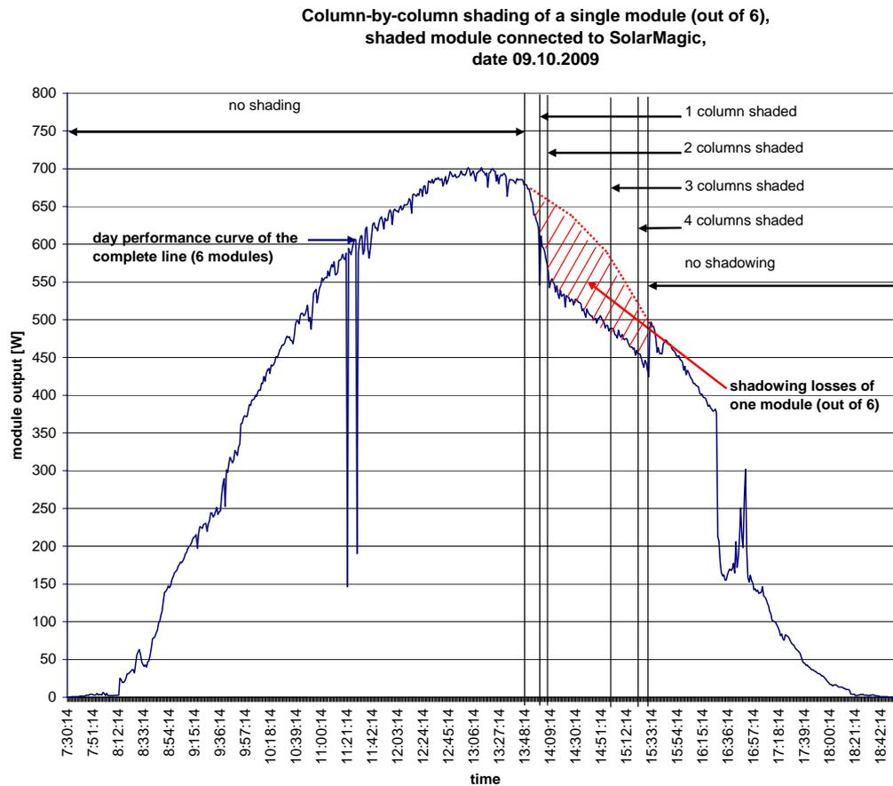
Fig. 10: column-by-column shading of a module connected to SolarMagic
