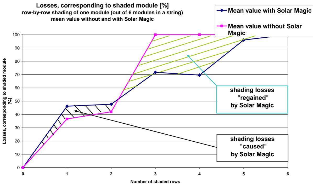
Fig. 13: Losses with row-by-row shading
