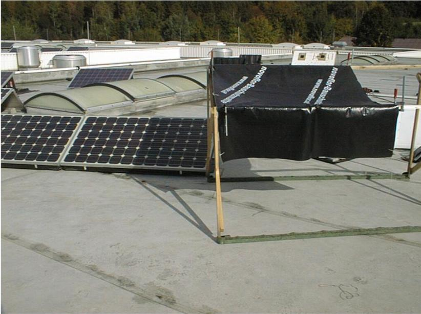
Fig. 5: Example of column-by-column shading
