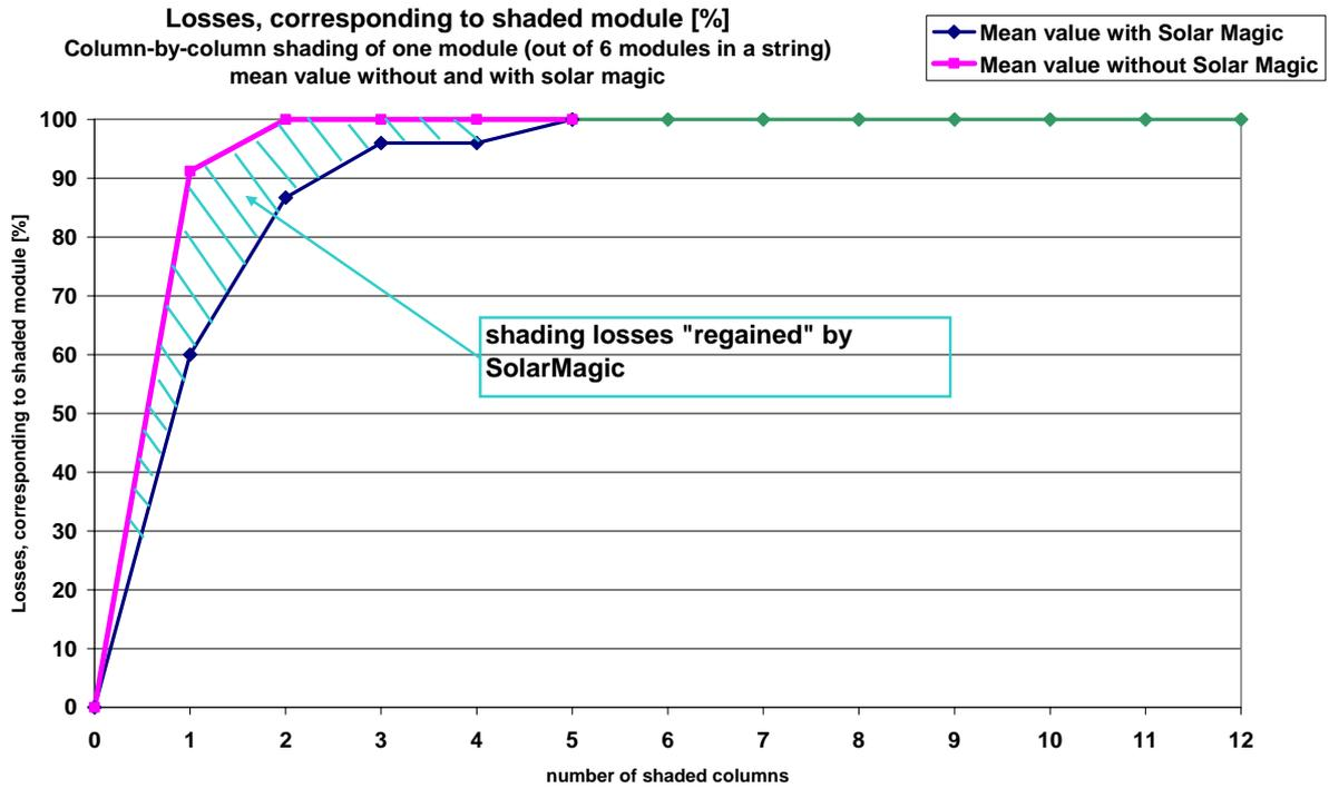
Fig. 12: losses with column-by-column shading
