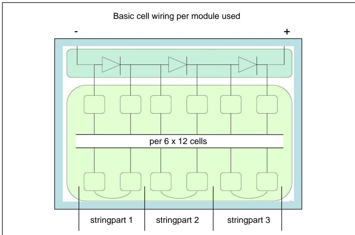
Fig. 2: interior cell wiring of one of the used modules
