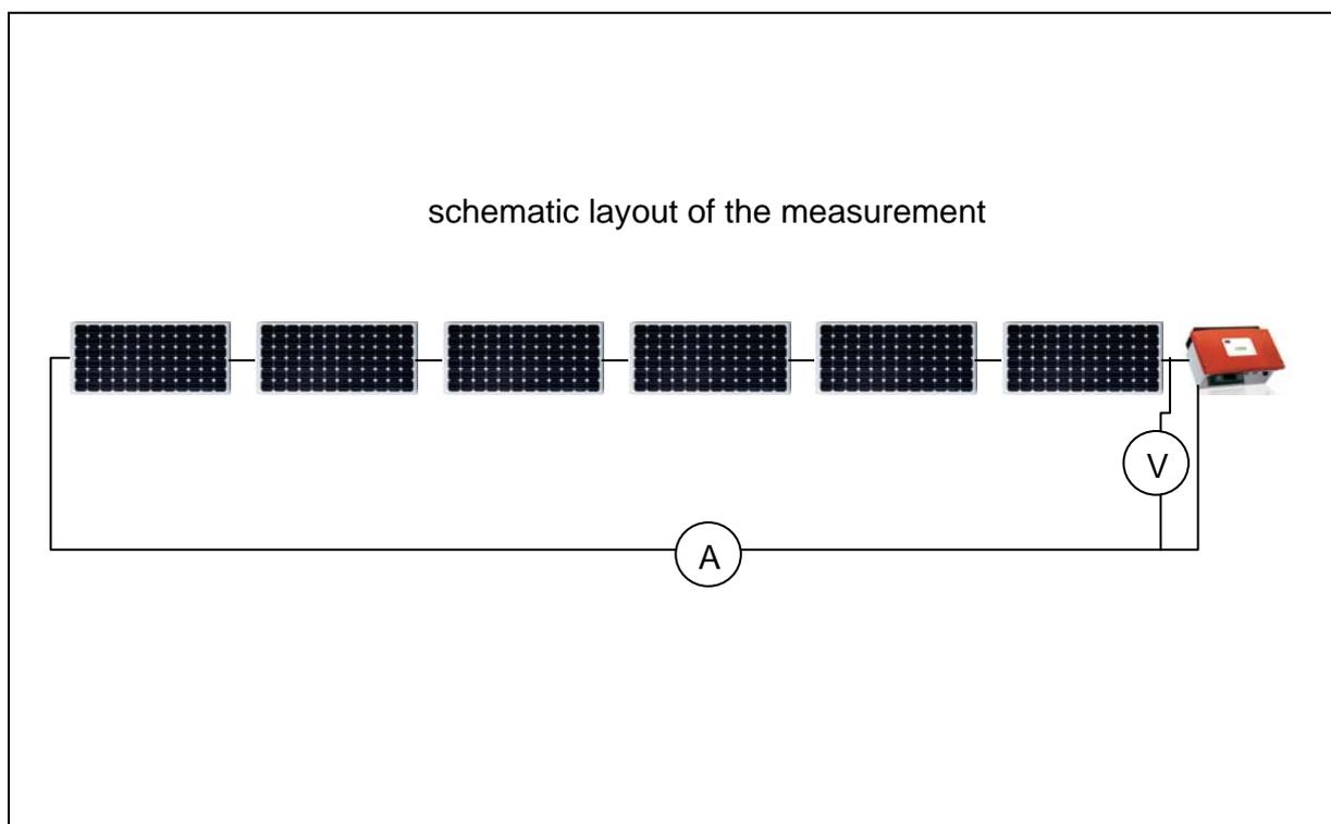
Fig. 1: schematic layout of the measurement wiring
