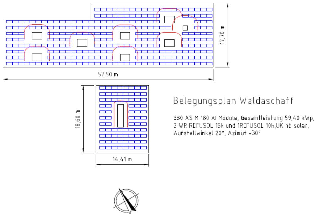
Fig. 6: Module array, disregarding the required distance of 1m (total output ca. 60 kWp)
