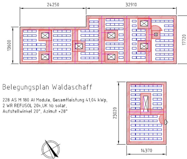
Fig. 5: Module array with the calculated, mandatory separation distance of 1 m.
