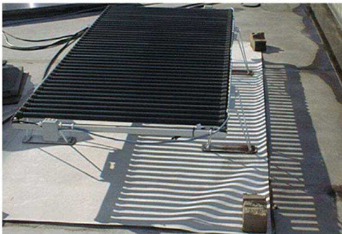
Fig. 4.: CIGS-cylinders cause partial shading of the reflector.
