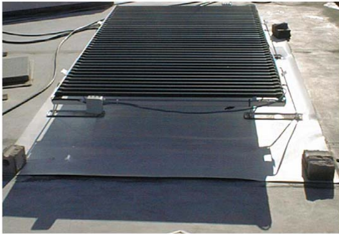
Fig. 5: CIGS-cylinders cause complete shading of the reflector.
